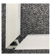
Insert the metal corners into the frame and push the pieces of frame together.
